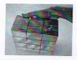
Fig 1: Picture of LiTraCon light transmitting concrete
